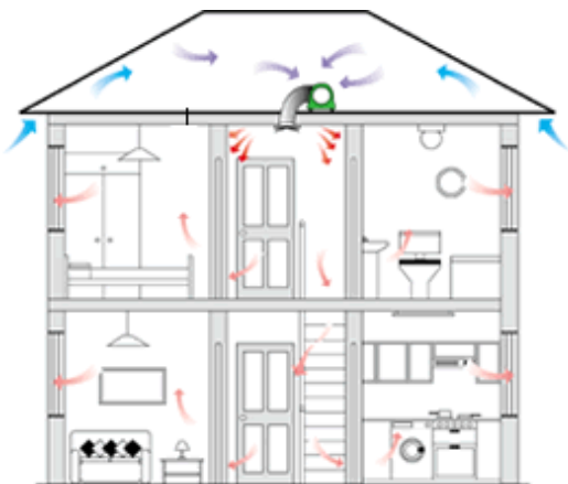
Typical Air-flow Distribution
